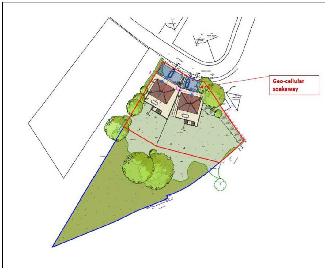
Figure 13: Proposed Drainage layout
